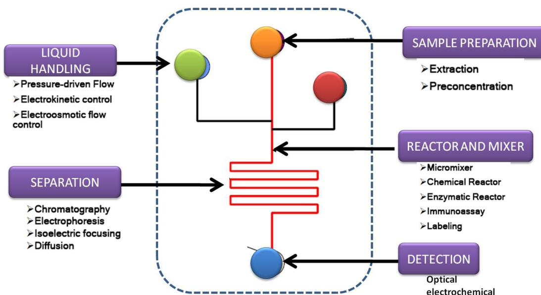
**Figure 2.** Components of diagnostic devices with a lab-on-a-chip approach
